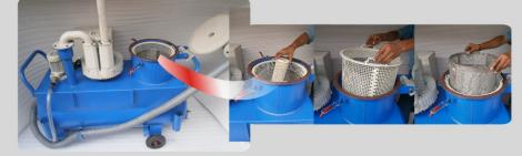
Sump Cleaner removes very fine dirt from Oil / Coolant upto 10µ & below by Vacuum created in the tank. There are no consumables hence no recurring cost. Collected dirt can be easily cleaned & the unit put back to use again
