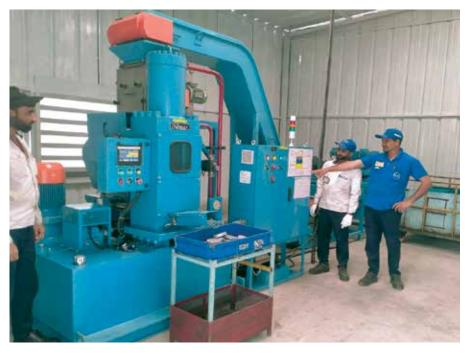
a dense briquette. This enables better melting yield and saving on electrical energy consumption in the furnace.
